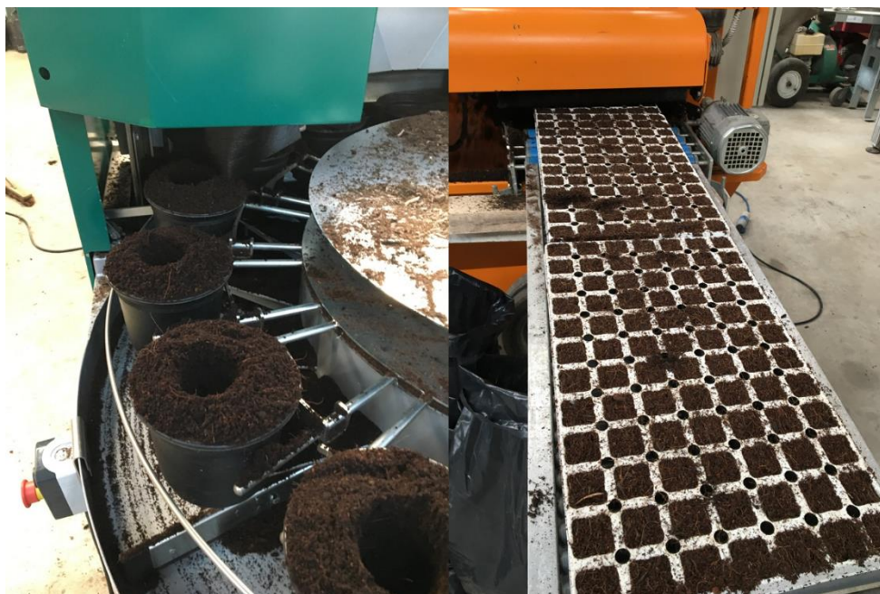
Figure 65. Testing prototype blends on a pot filling machine (2 L pots) and a tray-filling machine (84-cell trays).
